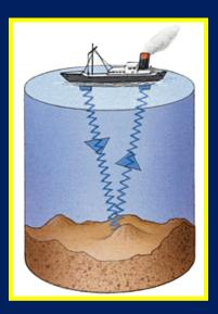
Sonar sends out sound waves and then measures the time it takes for sound waves to return.
