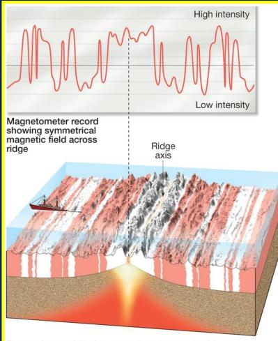
Research vessel towing magnetometer across ridge crest
