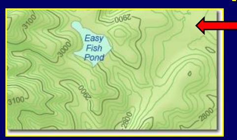
When the contour lines are spaced far apart, the elevation is changing very slowly and the terrain has gentle slopes.
